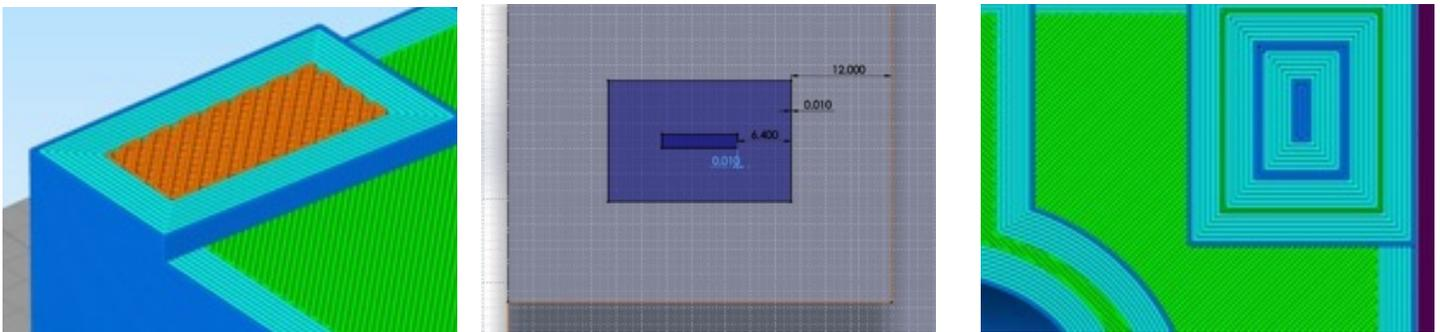
Using traditional manufacturing methods, an aluminum mold like the example above would cost \$20,000-\$25,000 and a four to five-week lead time. To produce this part with Essentium HTN-CF25, it would take five days to print and three days to post-process, getting the lead time down to just under two weeks. As for cost-savings, with ~\$5,000 for material, ~\$3,500 for post-processing, and ~\$3,000 for print time, the total cost of the product order would be ~\$12,000.
