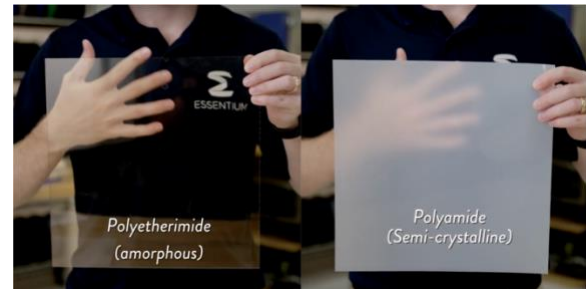
Figure 4. Optical clarity of an amorphous sheet of plastic vs. a semi-crystalline sheet.
